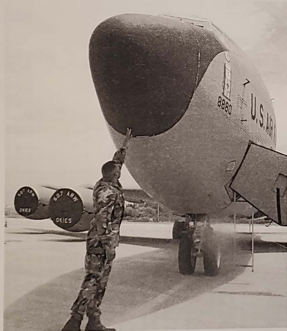
Air Force Reserve Airman Ron Arredondo visually inspects a new Weather Master radome installed on one of our Wing KC-135R Stratotankers. Arredondo was part of the team supporting the Oklahoma City Air Logistics Center's fit test and final Time Compliance Technical Order installation kit proof for the new radome.
