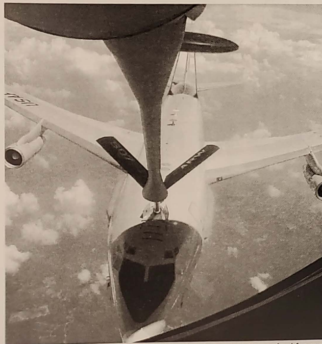
An E-3A from the 552 Air Control Wing hooks up to take on fuel from a unit KC-135 during the return flight home.
