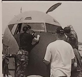
A 507th Maintenance team installs a new radome on a unit Stratotanker. See related story on page 6.
